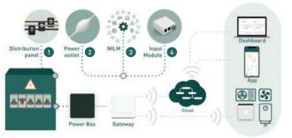
Or, use the Smappee Input Module to count pulses of sensors, meters and other devices or to monitor state changes (low/ high) to trigger other processes.
